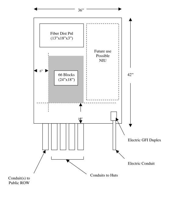
Note: Customer to provide plywood backboard for equipment mounting internal to NEMA box.
